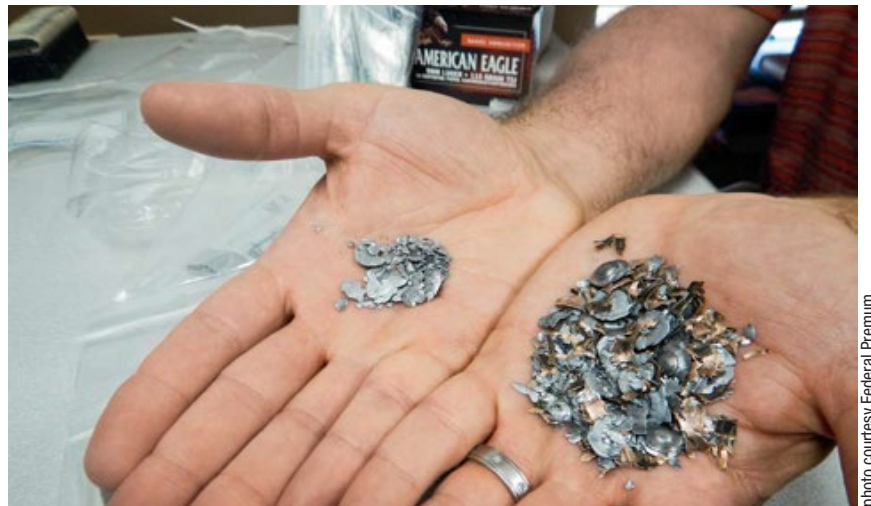
▲ Federal tested Syntech against jacketed bullets on steel targets to demonstrate how much less splashback Syntech (l.) produces.
