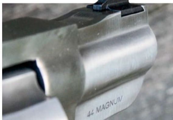
▲ The diminutive 2.75-inch barrel is tipped with a red-ramp front sight for good visibility in low light. Accuracy was more than acceptable.
