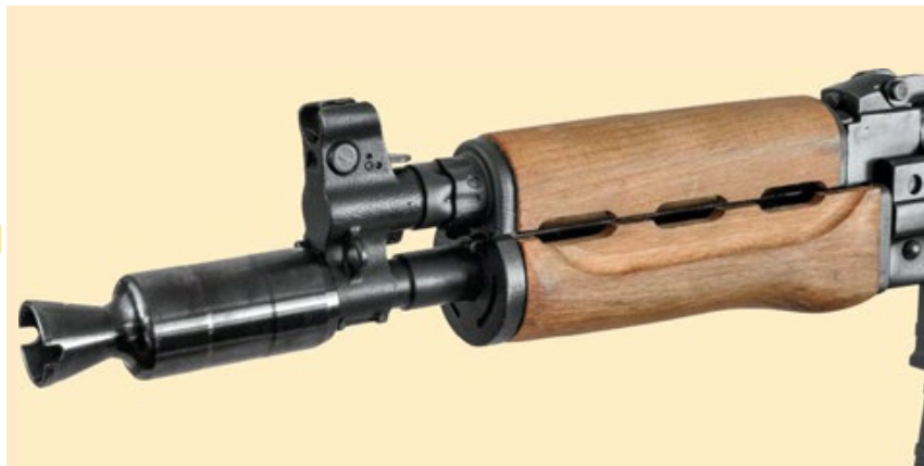
▲ The Zastava’s distinctive muzzle device works more as a pressure chamber to ensure reliability than as a flash hider.
