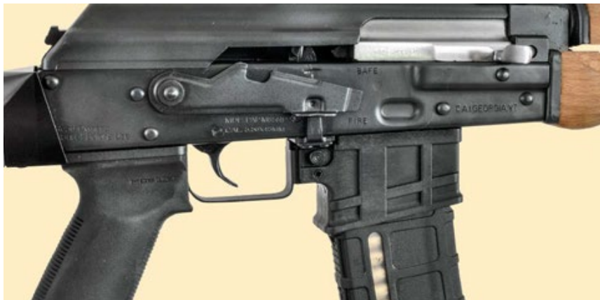
▲ The Zastava’s polymer magazine well allows it to be fed by standard AR-15 magazines. The safety incorporates a bolt hold-open notch.
