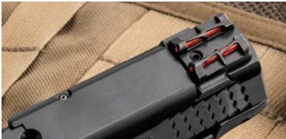
▲ Von Benedikt likes the visibility provided by fiber-optic sights but is suspicious of them on carry guns. Those on the Ported Shields calmed his fears due to the robust frame protecting the rods.
