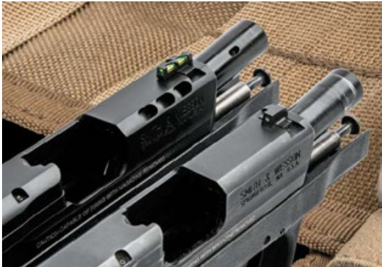
▲ The ported Shield 9mm exhibited a touch less recoil than the standard version with some loads; it’s likely the difference would be felt more with the .40.
