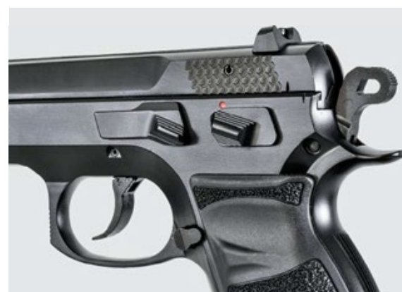
A The T-100 has a half-cock notch, which provides an alternative to cocked-and-locked carry and reduces both weight and trigger travel on the DA pull.
