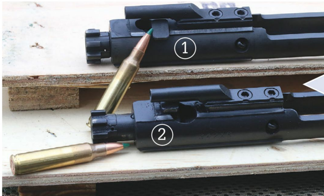
Two BCM bolts/carriers showing critical areas to oil ARs: circumference of bolt and cam pin/hole. Bolt number 1 was run bone dry and was getting slightly sluggish at 100 rounds. Bolt number 2 is well lubed, several hundred rounds in, and good for many more hard days.
