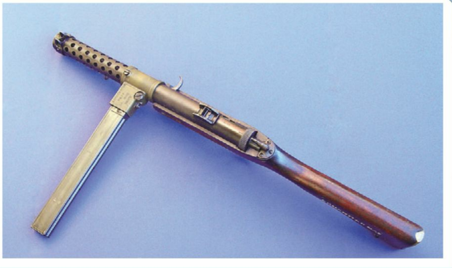
Above: Right side of Lanchester shows brass buttplate, magazine housing, and safety notch into which bolt can be rotated.
