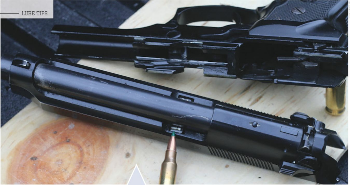
M9 gets best use of lube applied to each lug of the locking block.
