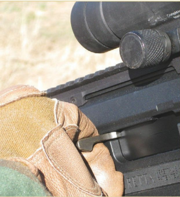
More robust extended charging handle would make ARX more user friendly.
