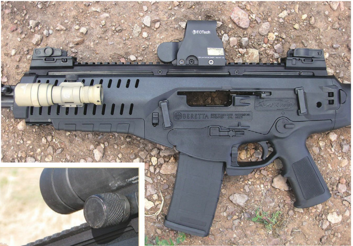
Above: Beretta ARX with EOTech optic attached to top rail and SureFire Mini Scout Light attached to left rail.
