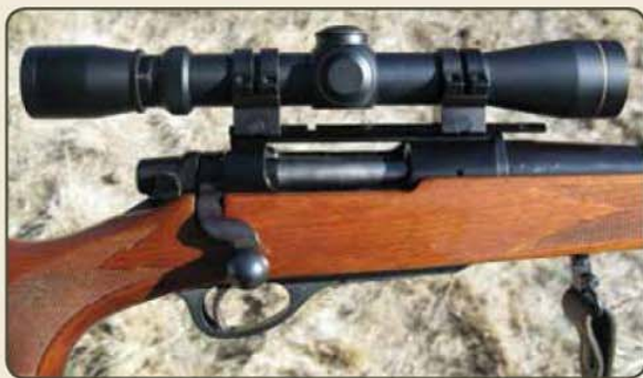
The Model 600 action (above) was derived from Remington's radical XP-100 pistol, and had the strange looking forward bent bolt. The Model 600 morphed into the Model 660 (below) beginning in 1968. While the Model 660 shares the same action with the 600, the Model 660 carbine was aesthetically improved and looked more like a conventional rifle.
