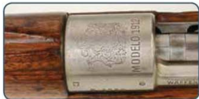
The actions of Chile's Model 1912 rifles were left in the white. They were made at Steyr, Austria.
