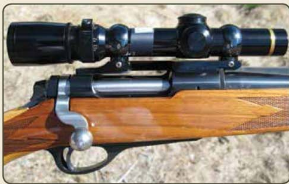
The Model 600 action (above) was derived from Remington's radical XP-100 pistol, and had the strange looking forward bent bolt. The Model 600 morphed into the Model 660 (below) beginning in 1968. While the Model 660 shares the same action with the 600, the Model 660 carbine was aesthetically improved and looked more like a conventional rifle.
