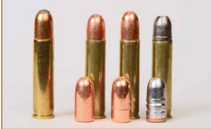
A Remington factory .351 WSL softpoint load (left) compared with Duke's handloads consisting of a 181-grain FMJ bullet of unknown make and its loaded round, a Buffalo Arms 181-grain FMJ bullet and loaded round and Duke's own 166-grain cast bullet from custom Accurate Mold and loaded round.
