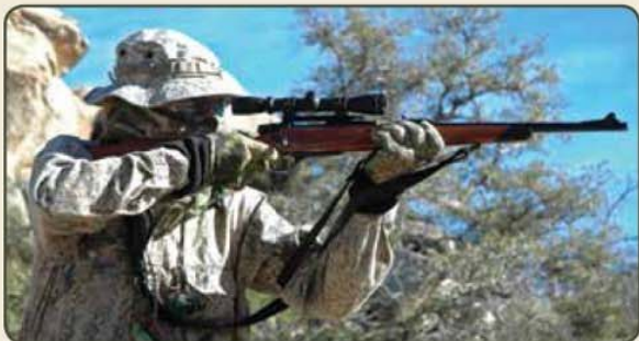
With its extra loop, the unique Ching sling is both a carry and a shooting sling. This is from Andy's Leather, and an extra swivel stud must be installed.
