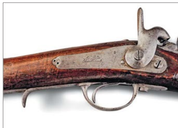
Markings on the 1840 back-action lock indicate it was manufactured at Châtelleraut. The spurred triggerguard is another of this arm's distinctive features.
